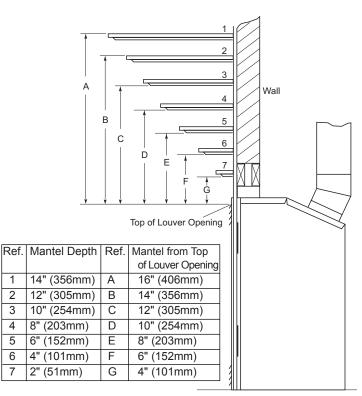
Figure 6 - Clearances for Combustible Mantels
